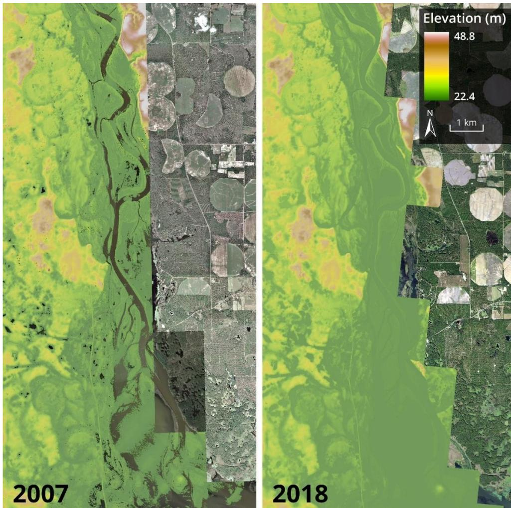
*Figure 12. DEMs of the Chattahoochee River delta generated using the 2007 (left) and 2018 (right) lidar surveys. Both DEMs are underlain by high-resolution National Agriculture Imagery Program (NAIP) aerial photographs taken close to the period of survey collection.*
