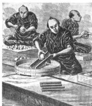
By permission of the "Scientific American." JAPANESE METHOD OF CHIPPING, GRINDING AND POLISHING ROCK-CRYSTAL BALLS.
