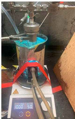
**Figure 2.3:** Light setup used for photocatalysis.
