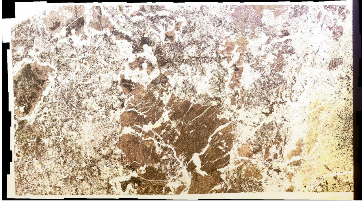
Figure S11. Thin section photo of PAV-2D-1 in PPL. Garnets are dark-brown to black and display patchy disseminated textures. Chlorite and serpentine are both clear, although serpentine is accompanied by fine-grained magnetite. Both pseudomorphed and precipitated diopside is brown.
