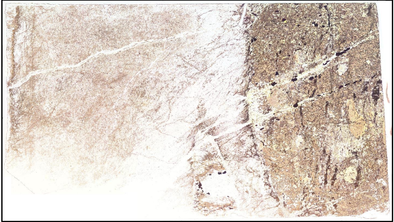
Figure S7. Thin section photo compilation of 21LAP-2Dc in PPL. Serpentine is clear to pale brown within the serpentinite and rodingite. Fine-grained chlorite is clear and pervasive within the serpentinite. Garnets are brown and do not display color variation. Diopside is present as pale brown hydrothermally precipitated grains (no pseudomorphed grains are present).
