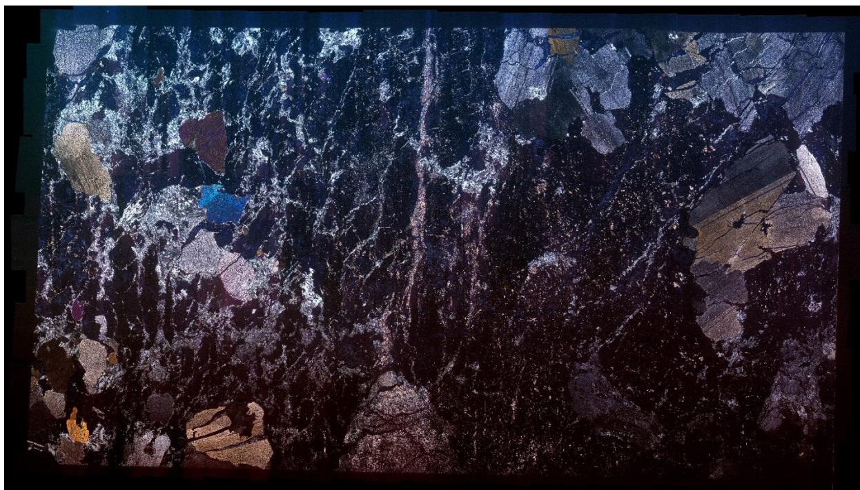
Figure S12. Thin section photo compilation of PAV-2D-2 in XPL, showing the interior of the Pavareto rodingite. The matrix is predominantly isotropic garnet with minor chlorite and serpentine. Psuedomorphed diopside displays first-order and second-order interference colors. Vein networks of diopside and chlorite have developed towards the interior of the rodingite and are overwhelmingly parallel to the contact. Minor amounts of hydrothermal titanite are present.
