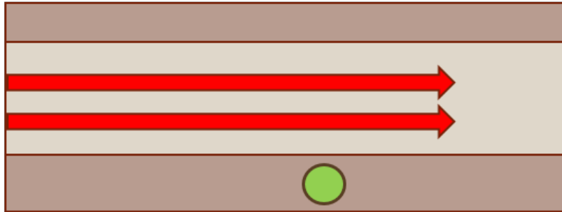
Figure 4.1: Cartoon of modulation doping, the light bring is the current channel and the green ball is the dopen, red arrow is the current flow.
