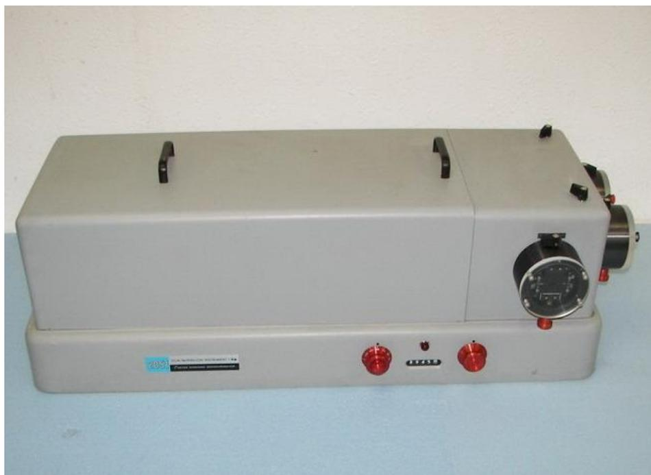
Figure 4. 5. McPherson model 2051 one-meter scanning monochromator
