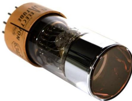
Figure 4. 6. photomultiplier tube Hamamatsu type R1387
