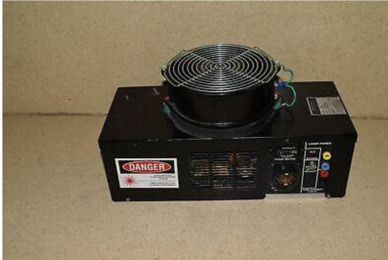
Figure 4. 2. Argon-ton laser system, Omnichrome model 532
