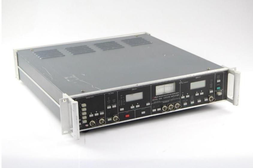
Figure 4. 12. EG&G Model 5201 Lock-in Amplifier
