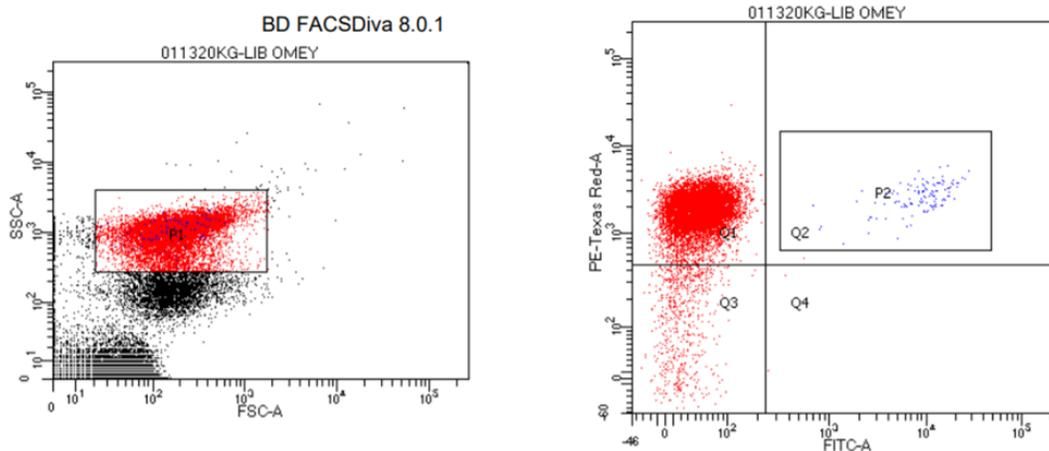
**Figure 3.9. FACS of the *EcTyr*-OMeYRS + *EcTyr*-pBPARS mock library.** The population of cells sorted were chosen based on their forward scatter and side scatter light ratio (left). The sorted cells were further scrutinized for their ratio of sfGFP (FITC-A): mCherry (PE-Texas Red-A) fluorescence. Parameters were outlined as quadrant 2 (Q2), resulting in the collection of only 1.1% of the total parent population (right).
