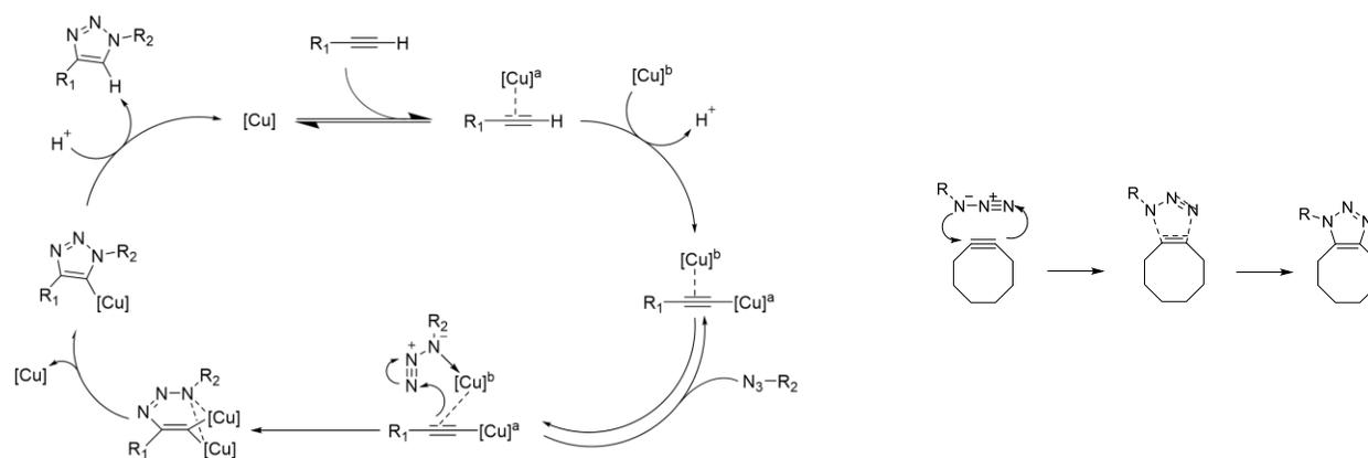
**Figure 4.4. Azide-alkyne coupling reaction mechanisms.**<sup>13, 14</sup> Copper-catalyzed azide alkyne cycloaddition is pictured left and strain-promoted azide alkyne cycloaddition is pictured right.
