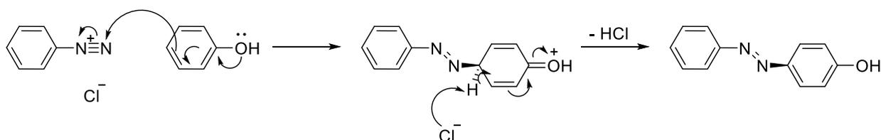
**Figure 6.8.** Azo-coupling mechanism between aryl diazonium ions and aromatic nucleophiles.
