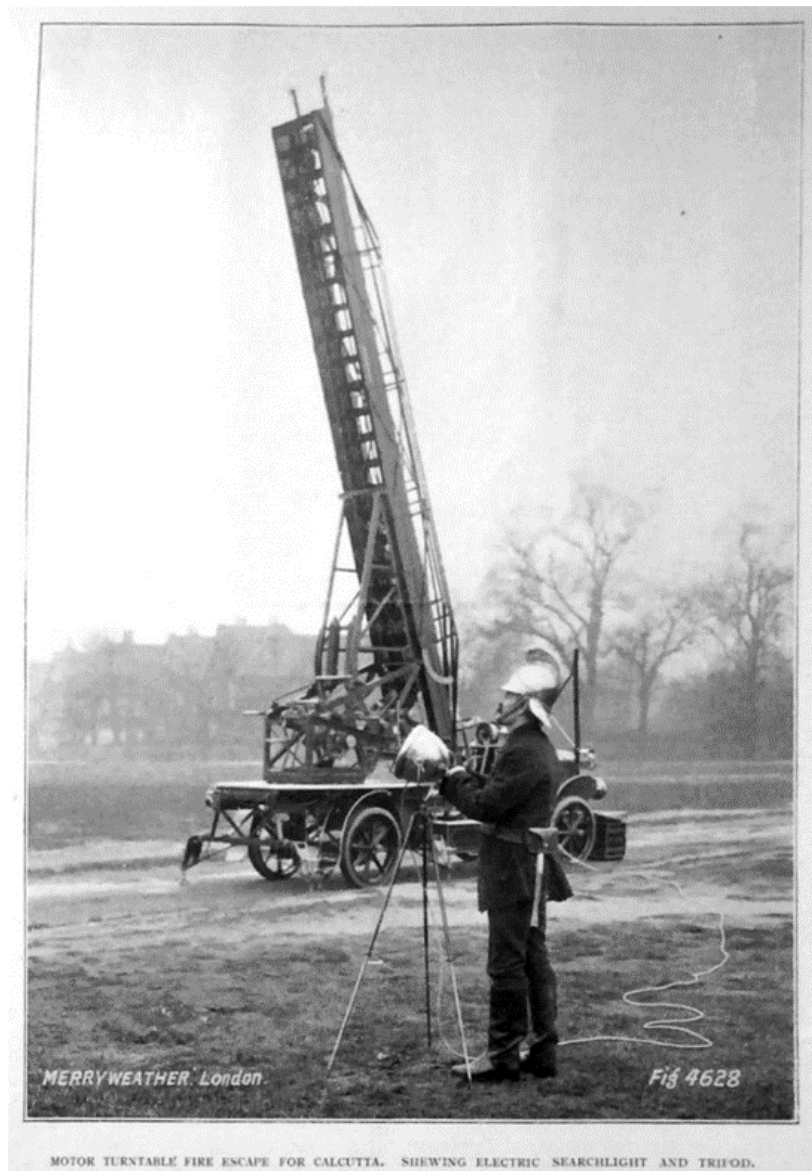
Figure 8 Petrol-motor turntable fire escape ladder for Calcutta from The Fireman (1914).
