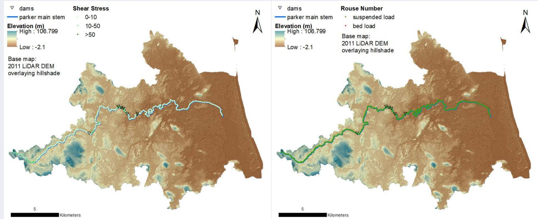
Most parts of the Parker River main stem have a shear stress between 0 and 10 Pa. Relatively higher shear stress is observed at the head water region where slopes are steeper and at locations of dam headwall.
