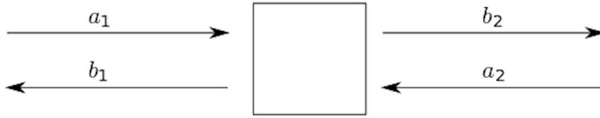
**Figure 1-2. A two-port system defining the S-matrix.**
