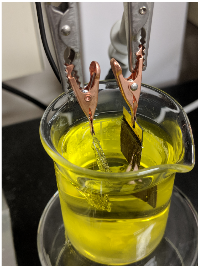
FIGURE 2.1: The two electrode setup for DENA. A platinum coil acts as a counter electrode, and the gold surface of the chip acts as the working electrode.
