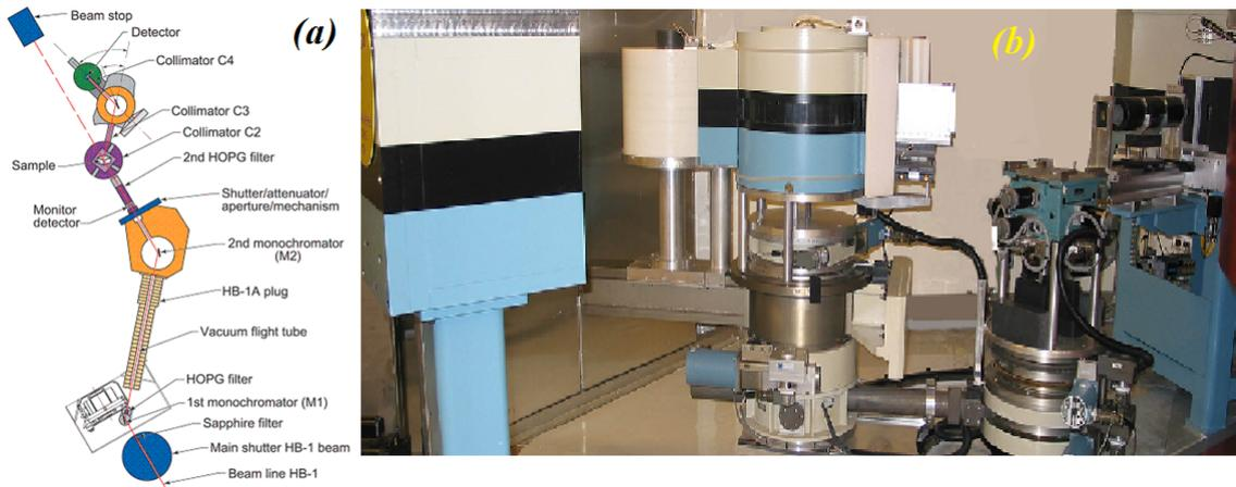
**Figure 3.12:** (a) Schematic of a triple-axis spectrometer at HB1A of Oak Ridge National Lab (ORNL); (b) Real image of HB1A. Adopted from [7].
