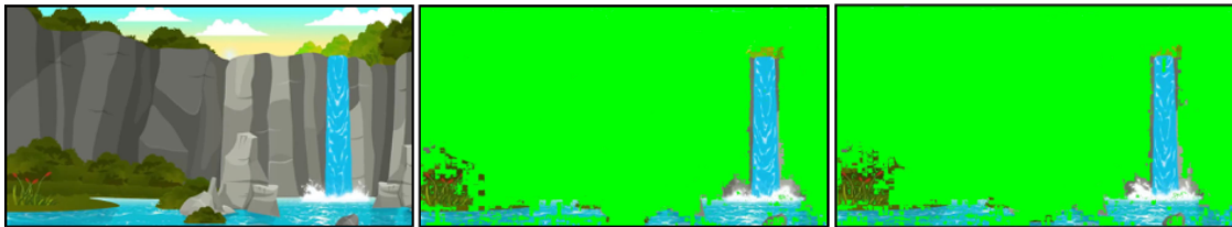
Figure 1. Example of .gif compression. Three frames of an animation are depicted. The waterfall flows, and the flowers in the bottom left corner sway in the wind, but most pixels in the image remain stationary. The image can be compressed by encoding repeated pixels as green space, meaning that only pixels that differ from their prior values need to be updated. In other words, in each frame, pixels only encode prediction error—the difference between the predicted and observed value for that pixel.
