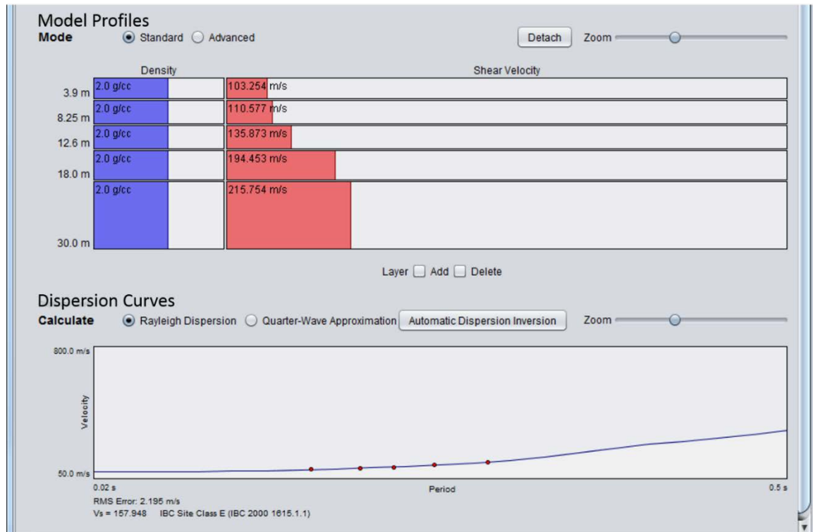
Figure 11: Example of forward modeling using ReMi. By clicking and dragging the Vs profile (vertical red shaded area in the “Model Profiles” panel) and the layer interfaces (horizontal black lines in the “Model Profiles” panel), the modeled dispersion curve (blue line in the “Dispersion Curve” panel) can be adjusted to overlay the dispersion picks (red filled circles). The RMS error (2.195 m/s) that is shown here is small enough to finish the forward modeling.
