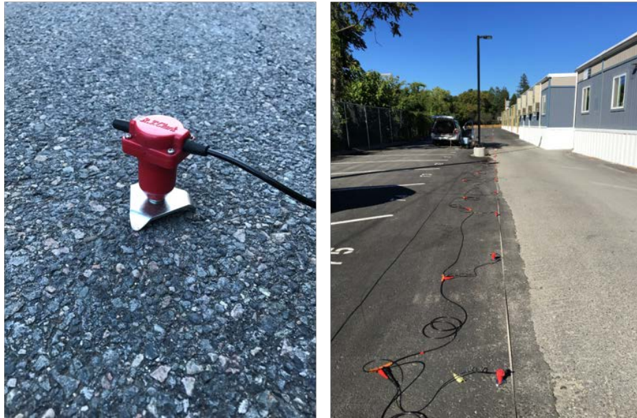
Figure 3: These are examples of geophones with spikes or tripods. (a) These photographs show a geophone with a spike base and a geophone with a tripod base. (b) Examples of the installation of a geophone with a spike base, where the spikes have been pushed into the ground. (c) Examples of geophones with tripods that have been installed on a paved surface.
