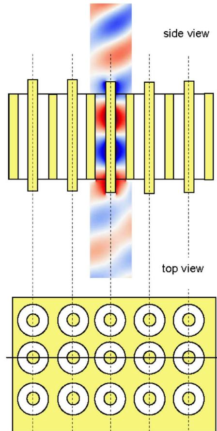
FIG. 2. (Color online) FDTD simulation of the transmission of light ( $\lambda=500$  nm) through a simple nanocoax medium. Film thickness is 800 nm, array period is 400 nm, diameter of the inner core of the nanocoax is 100 nm, and the inner diameter of the outer electrode is 300 nm. At bottom is a top view.
