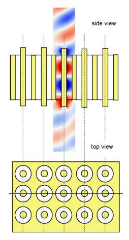
FIG. 2. (Color online) FDTD simulation of the transmission of light ( $\lambda$ =500 nm) through a simple nanocoax medium. Film thickness is 800 nm, array period is 400 nm, diameter of the inner core of the nanocoax is 100 nm, and the inner diameter of the outer electrode is 300 nm. At bottom is a top view.
