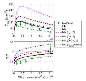
**Fig. 5.** The modeled result of  $C_{OA}$  and O : C from both the original model (OM, denoted by solid lines) and modified model (MM, denoted by dash lines) (Murphy et al., 2012a; Donahue et al., 2012a) with the initial  $\alpha$ -pinene of 281 µg m<sup>-3</sup> when some parameters are varied (see legend).
