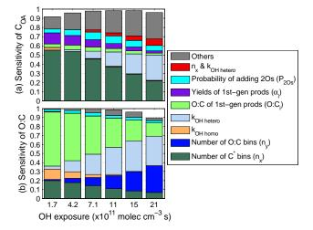
**Fig. 7.** The sensitivity of modeled (a)  $C_{OA}$  and (b) O:C for the six cases that represent the evolution of SOA at different OH exposure levels of  $(2-20) \times 10^{11}$  molec cm<sup>-3</sup> s. Only important model parameters (sensitivity greater than 0.05 for at least one case) are shown here.
