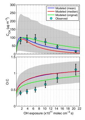
**Fig. 6.** The variation of modeled  $C_{OA}$  and O: C resulting from the variation of model parameters of the base-case original model for the case with initial  $\alpha$ -pinene of 281 µg m<sup>-3</sup>. The gray shadow extends to the most extreme data points corresponding to 97.5 and 2.5 percentiles, that is, 95% coverage of the data. The error bars show the uncertainties of measured  $C_{OA}$  and O: C.
