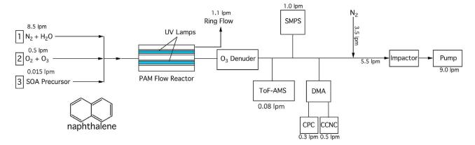
**Figure 1.** A schematic of the experimental setup for SOA sample generation and collection adapted from *Lambe et al.* [2011a]. As indicated, input lines 1 and 2 provided carrier gases (N<sub>2</sub> and O<sub>2</sub>) and OH radical precursors (O<sub>3</sub> and H<sub>2</sub>O). Line 3 provided naphthalene precursor to generate SOA. (lpm represents liter per minute).
