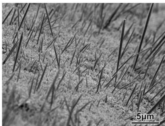
Figure 2.6 SEM image showing the binary growth of both long and short NWs on defect-rich deformed areas of the Cu foil. Reprinted with permission from ref. 1, © 2010 Wiley-VCH.
