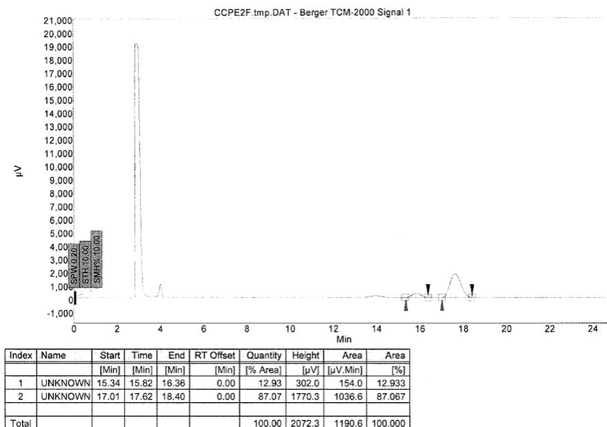
**Table 2.1, Entry 3:** 2-Phenylprop-2-en-1-ol (**1.43**) was hydroformylated using *p*-toluenesulfonic acid (396  $\mu\text{L}$  of  $5.69 \times 10^{-4}$  M in benzene,  $2.25 \times 10^{-4}$  mmol, 0.15 mol%) at 400 psi CO/H<sub>2</sub>. The branched product was isolated in 78% yield and 69% ee.
