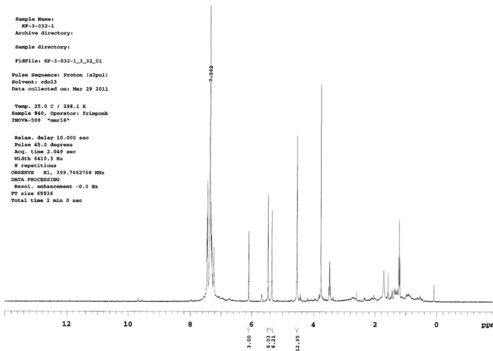
**Table 2.4, Entry 2:** 2-Phenylprop-2-en-1-ol (**1.43**) was hydroformylated using *p*-toluenesulfonic acid (132  $\mu$ L of  $5.69 \times 10^{-4}$  M in benzene,  $7.5 \times 10^{-5}$  mmol, 0.05 mol%) at 400 psi CO/H<sub>2</sub>. Analysis of the crude reaction mixture showed a 58% conversion by <sup>1</sup>H NMR. The branched product was isolated in 13% yield and 11% ee.
