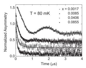
FIG. 4. Low-temperature depolarization curves for samples with  $x=0.0017,\,0.0085,\,0.0406,\,$  and 0.0854 (muon polarization parallel to the c axis). Solid lines are fits to Eq. (2);  $G_{\rm F\mu F}$  (t) = 1 for  $x\geqslant 0.0085$ . The curves have been offset for clarity.
