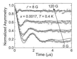
FIG. 5. Measured (open squares) evolution of the muon depolarization with increasing longitudinal field at low temperature and simulated (solid lines)  $F\mu F$  data over the same field range with magnetic disorder  $\Gamma=8$  G.
