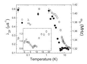
FIG. 2. Temperature dependence of the fit parameters  $\lambda_{ZF}$  (left axis),  $\omega_D$  (right axis), and  $\beta$  (inset) for the x=0.0017 sample (muon polarization parallel to c axis).
