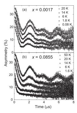
FIG. 1. Temperature evolution of the depolarization curves for samples with (a) x = 0.0017 and (b) x = 0.0854. Solid lines are fits to Eq. (2). In (b)  $G_{F\mu F}(t) = 1$  for the curves at T = 1.6 and 6 K. In (a) the curve for T = 50 K would be nearly identical to T = 20 and 14 K. Curves have been offset for clarity.
