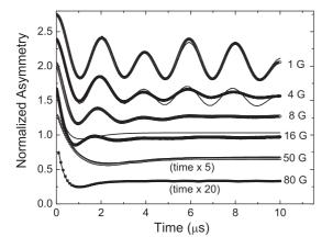
FIG. 3. Simulated evolution of the F $\mu$ F depolarization with increasing magnetic disorder  $\Gamma$ . Simulated data (symbols) are fitted with (solid lines) Eq. (2) for 1 and 4 G, and Eq. (3) for 16, 50 and 80 G.
