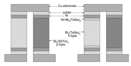
FIG. 1. Both (a) and (b) show one p-n couple that can be used as a thermoelectric generator or Peltier cooler. Typical TE devices contain many couples. The ideal solder connection to the Ni diffusion barrier for a  $Bi_2Te_3$  p-n couple is shown in (a) where the Ni does not diffuse into the TE material. (b) The actual case during fabrication and operation where the Ni diffuses into the n-type TE material which is believed to be the cause of device degradation.<sup>4</sup>
