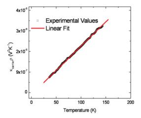
FIG. 6. (Color online)  $\kappa_{\text{carrier}}\rho$  is plotted against temperature from 35 to 150 K. The black points represent the measured data, while the red line is the linear fit. The slope of the linear fit provides the Lorenz number  $L = 2.21 \times 10^{-8} \text{ V}^2 \text{ K}^{-2}$ , and the *y* intercept gives  $\kappa_{\text{lattice}} = 2.14 \text{ W mK}^{-1}$ .
