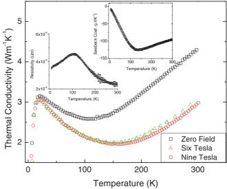
FIG. 5. (Color online) Thermal conductivity is plotted against temperature at magnetic fields of 0, 6, and 9 T for  $Bi_{0.88}Sb_{0.12}$ . The top right inset plots the Seebeck coefficient against temperature, while the top left inset plots *r* vs *T* from 5 to 300 K in zero magnetic field. It can be clearly seen that the bipolar contribution to the Seebeck coefficient becomes non-negligible around 150 K.
