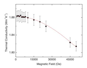
FIG. 4. (Color online) Thermal conductivity is plotted against magnetic field from 0.1 to 5 T and fit using Eq. (8) and  $\mu_d$  from Fig. 3. It is found that  $\kappa_{\text{lattice}} = 1.29 \text{ W mK}^{-1}$ .
