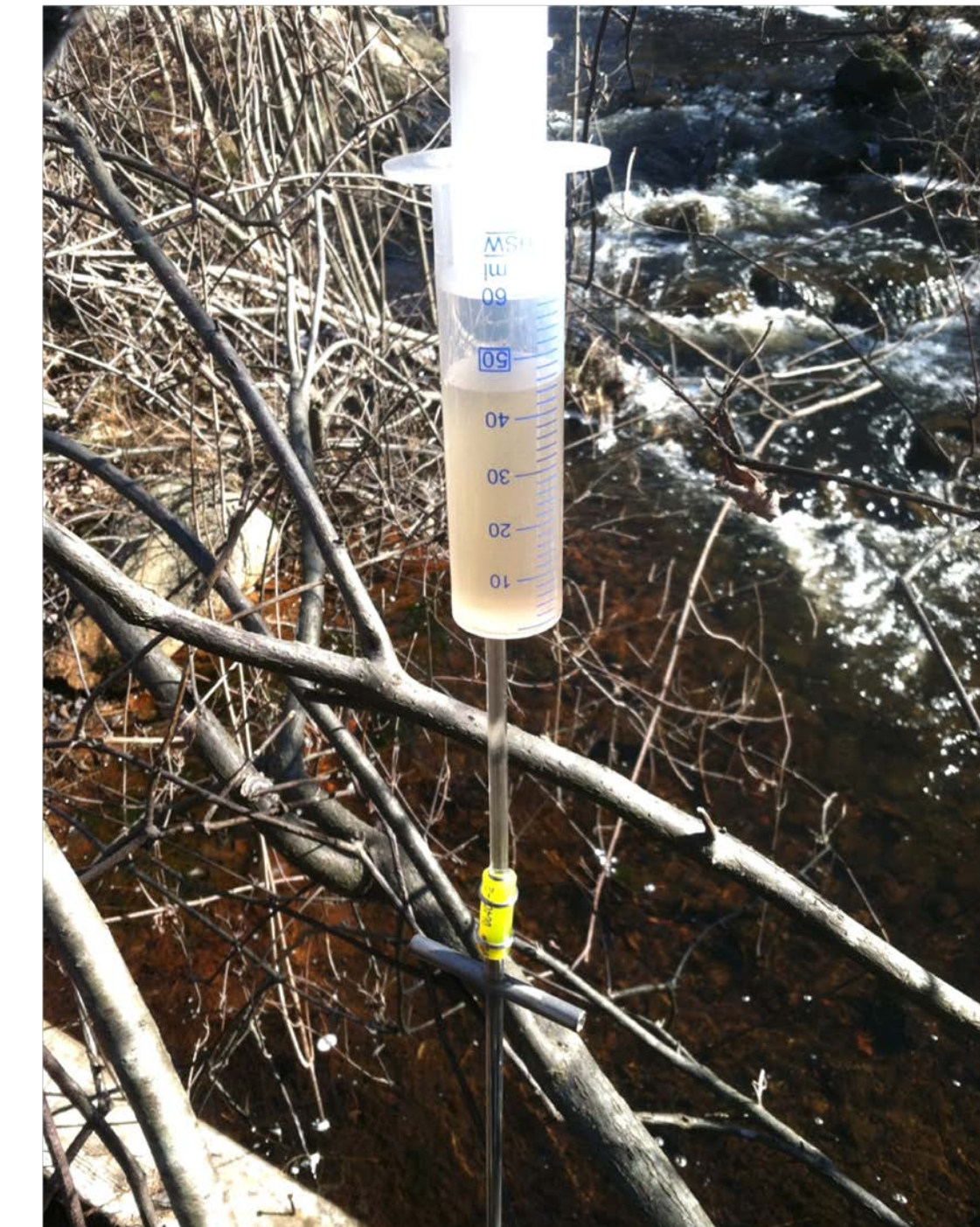
Fig 4. Photo of groundwater being extracted using the pushpoint sampler.
